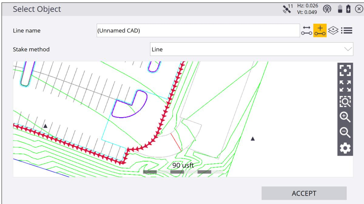
3. If necessary, before confirming the selection, change the line direction using the
