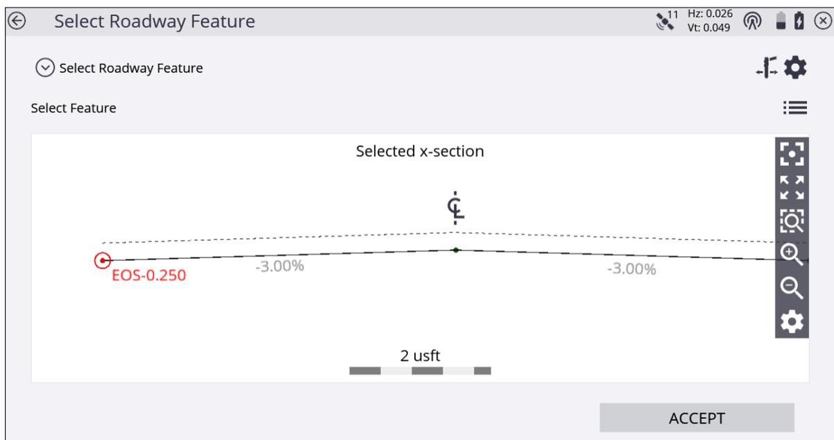
If you are navigating up station, the normal cross section view is displayed left to right as expected. If however, you are navigating down station, then the cross section would
