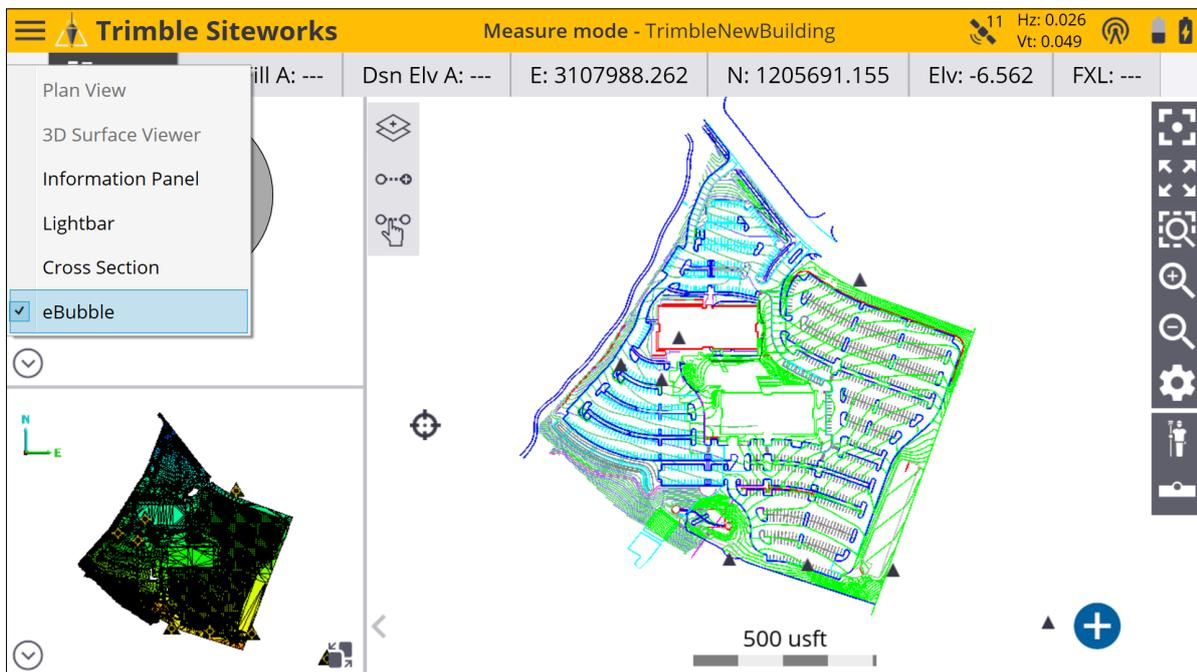
To display the data from the top and bottom side panels, select the **panel switch** icon in the bottom right of these small panels:
