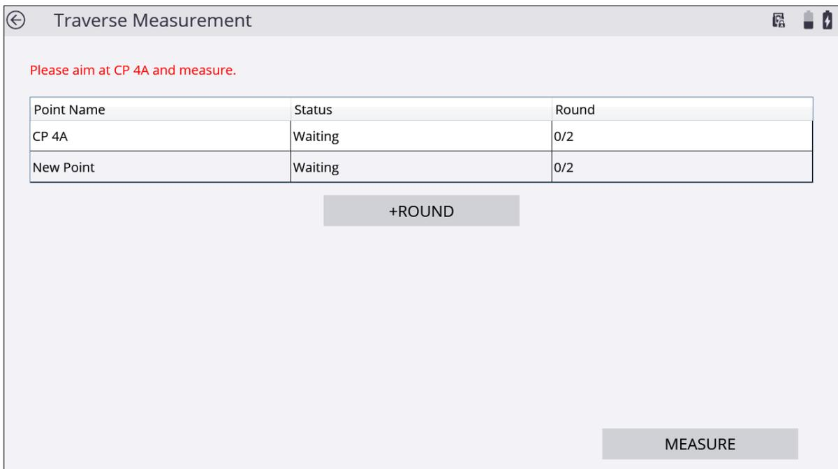
9. Repeat Step 3 through Step 7 to create traverse measurements at all required stations and complete building the traverse.
