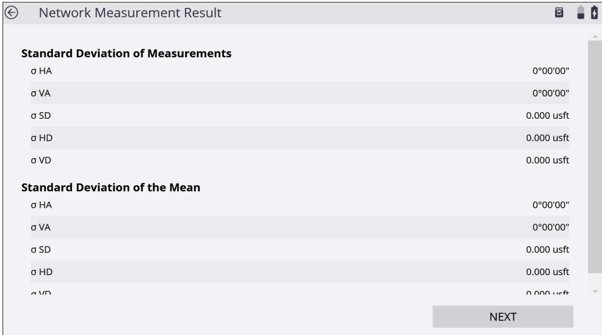
17. The next screen shows the differences between the measured rounds for each target:
