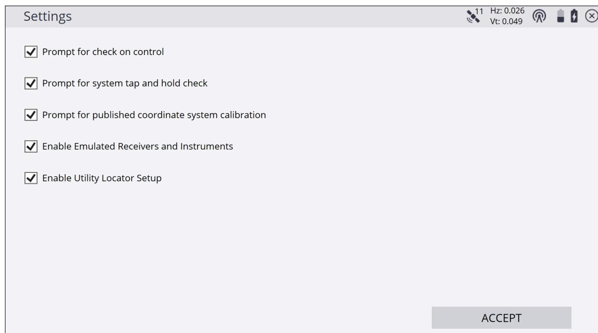
After the **Enable Utility Locator Setup** check box is selected, tapping the **Home** menu, **Measure** shows a new menu item for utility locator setup.
