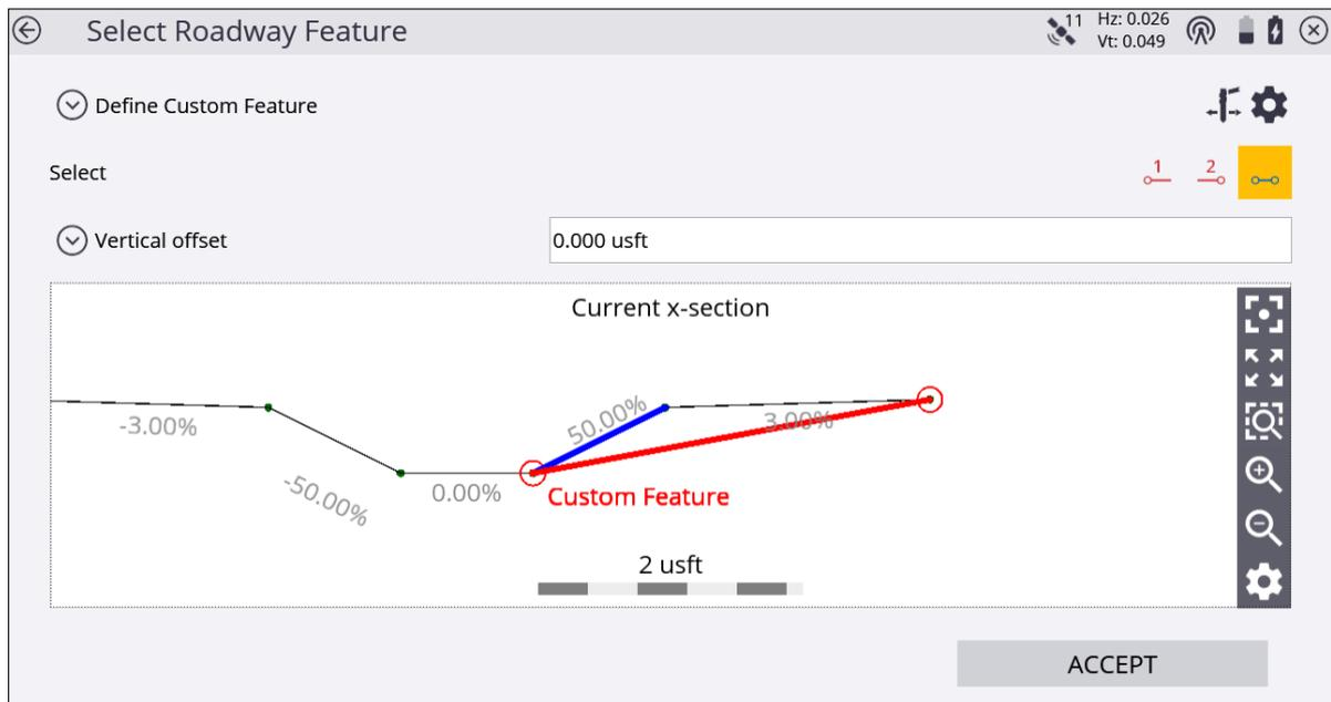
2. Select two feature nodes that will form the subgrade. You can access subgrade adjustments of the finished grade from the map view during stakeout or by tapping on the Road Settings gear icon in the upper right side of the screen (access the **Road** settings through **Settings**, and then enter the amount and direction for the offset).
