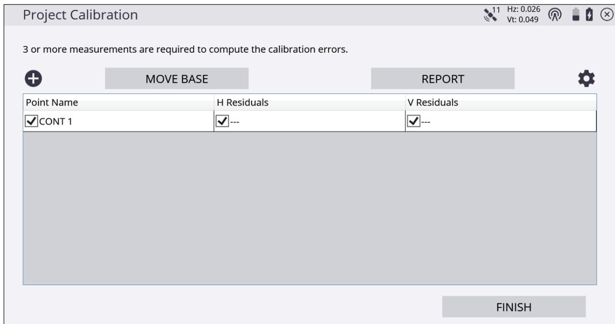
4. When enough control points have been measured, horizontal and vertical residuals will appear on the screen.
