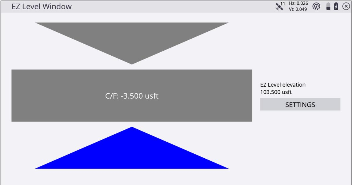
To re-enter the settings window to change the EZ Level elevation and/or measure a new benchmark elevation, tap **SETTINGS**.
