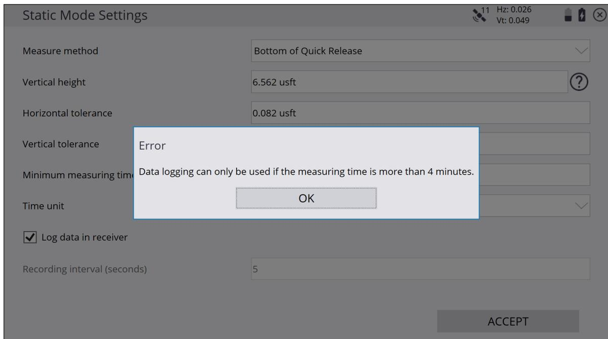
5. Complete the options for the antenna height, how long you want to measure for, and select whether or not to store the raw data in the receiver. You need to measure at least four minutes to store RAW data in the receiver, which can then be used for postprocessing.
