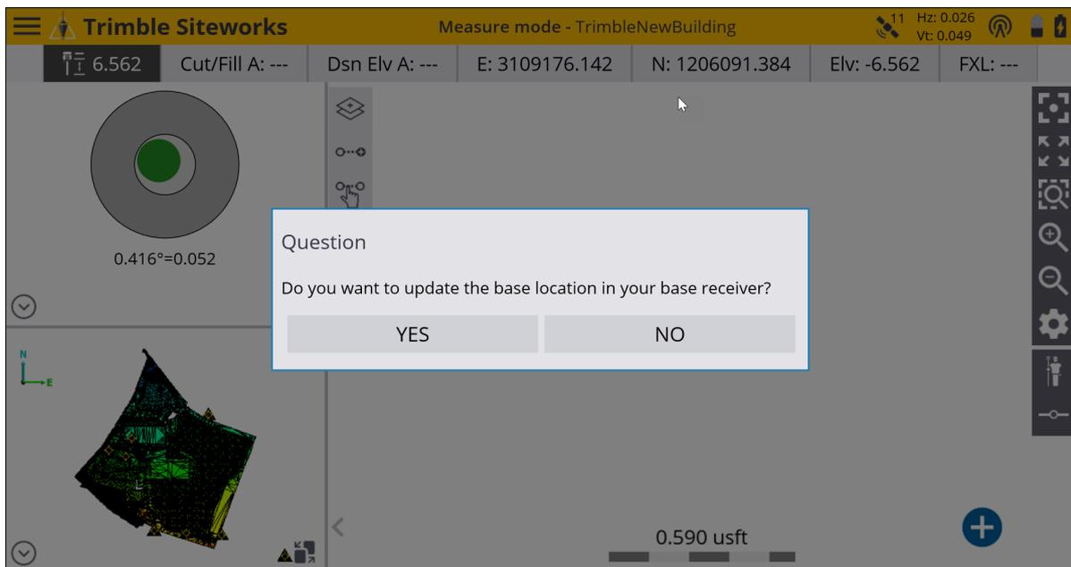
Selecting **Yes** will enable an update of the location of the base receiver from its autonomous position to its true RTK-calculated location. This is now the equivalent of having a traditional base setup on a known control point.
