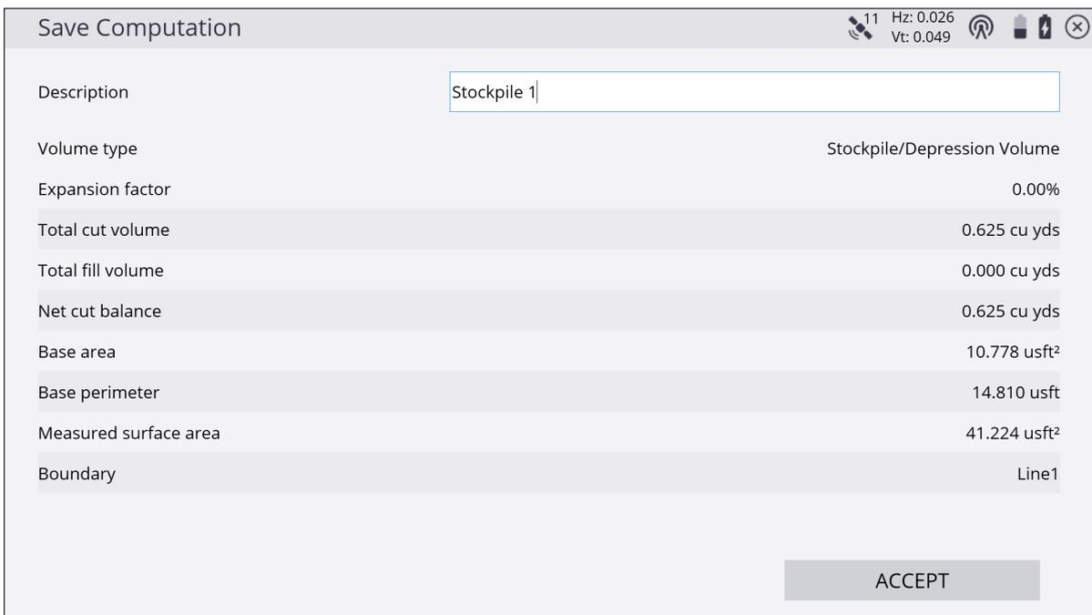
The results of the volume calculation are stored in the TaskLog.txt and can be reviewed using the name of the volume in the system log, accessed via **Data Management / Log**.
