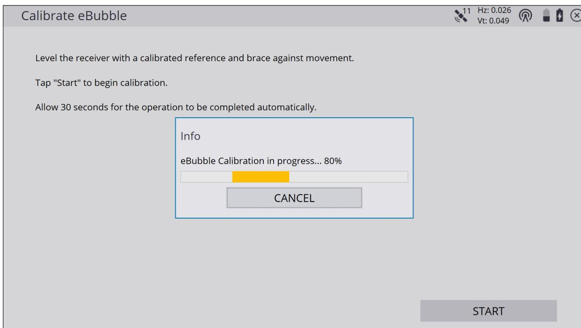
After the calibration is complete, a message appears indicating the finished calibration. The receiver’s front panel must be facing you for correct operation, as the eBubble’s movements and display within Siteworks are oriented based on the receiver’s front panel facing the operator. When mounting and using the receiver in vehicle mode, the front panel should be oriented towards the rear of the vehicle .
