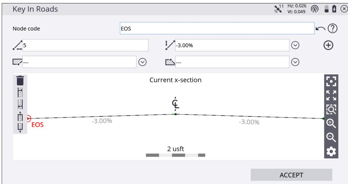
Copy the right side of the road over to the left side by tapping the copy template button. When the template is complete, tap **Accept**. Enter a name for the template and whether you want to store the template in a library that can be accessed from any site on the controller.
