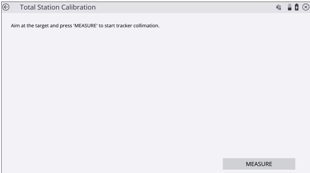
**NOTE** – There can be two reasons for significant change between old and new values: (1) The total station has received a knock or bump in transit that may need a service correction, or (2) there has been an observation error.
