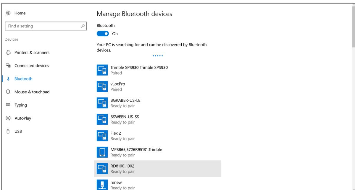
2. After the Radiodetection locator appears in the device list, click on it to begin the pairing process. Enter **1234** for a pairing code and tap **Next**.
