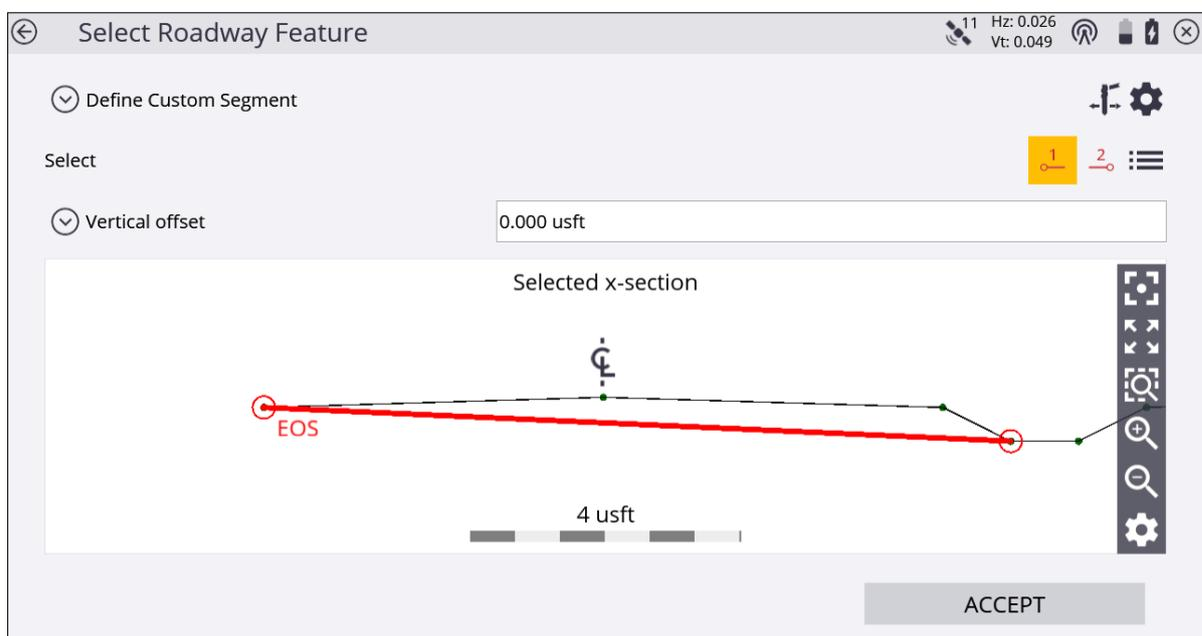
3. You will get guidance to the first point you have selected. Stake out this point as usual. You can also specify a horizontal offset for the stake the same way as for a normal roadway feature. You can also enter a random offset and apply the grade of the roadway and then stake this layer infinitely to the left or to the right and get the cut/fill to this segment.
