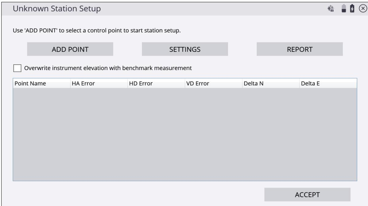
3. Select a point on the map by tapping directly on it and entering the name into the text box, or from the list, by tapping
