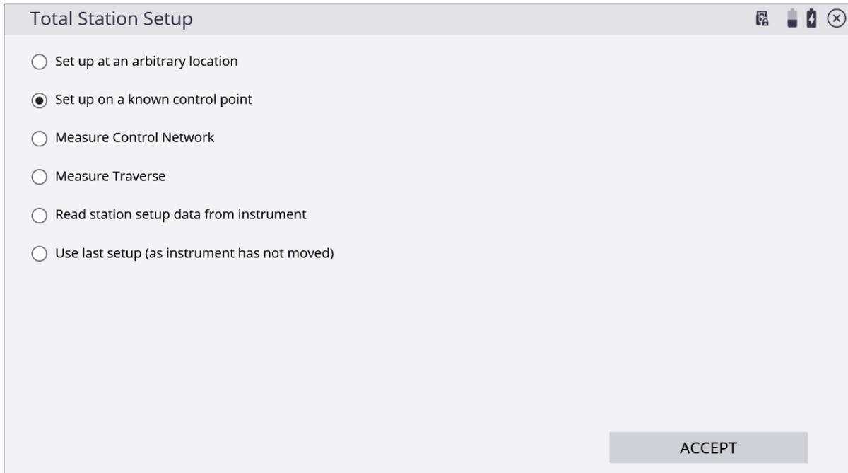
2. Select the instrument's location point by tapping directly on it and entering the name into the text box, or from the list, by tapping
