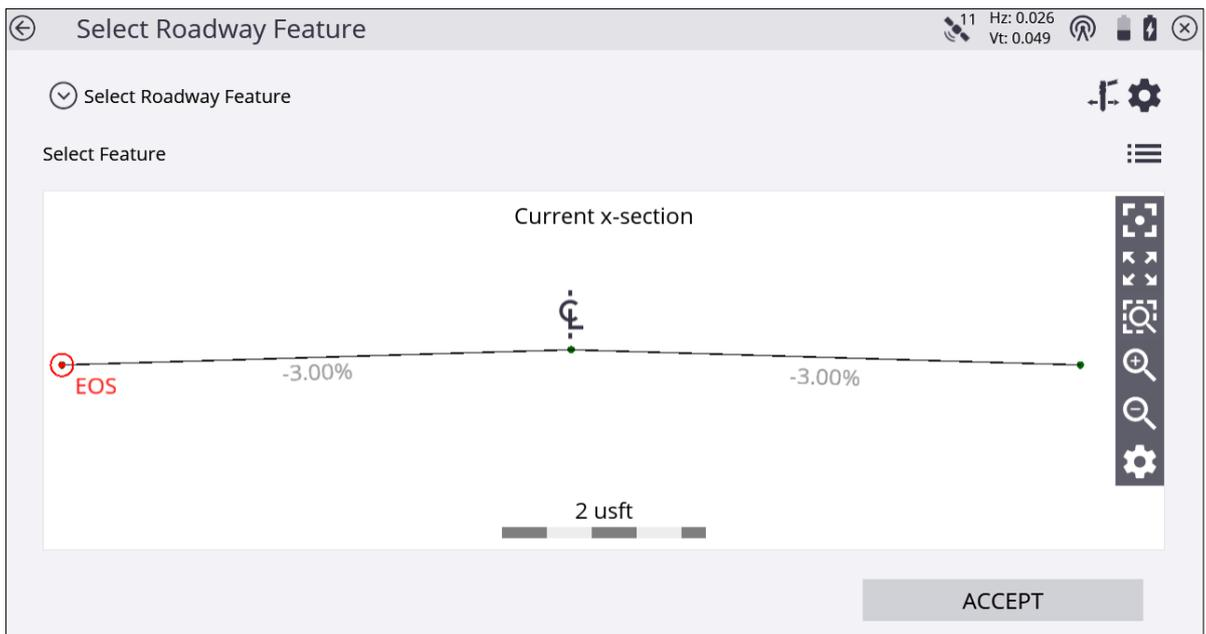
If the node is on the finished grade model, the name of the node would be ER, for example. If the node being selected is on the subgrade adjusted surface, it would be named ER-0.250; meaning it is the ER node, but it has a -0.250 m offset. A subgrade can be entered by accessing Road Settings through **Settings/ Roads** or by tapping the Road Settings icon in the upper right side and entering a subgrade offset value.
