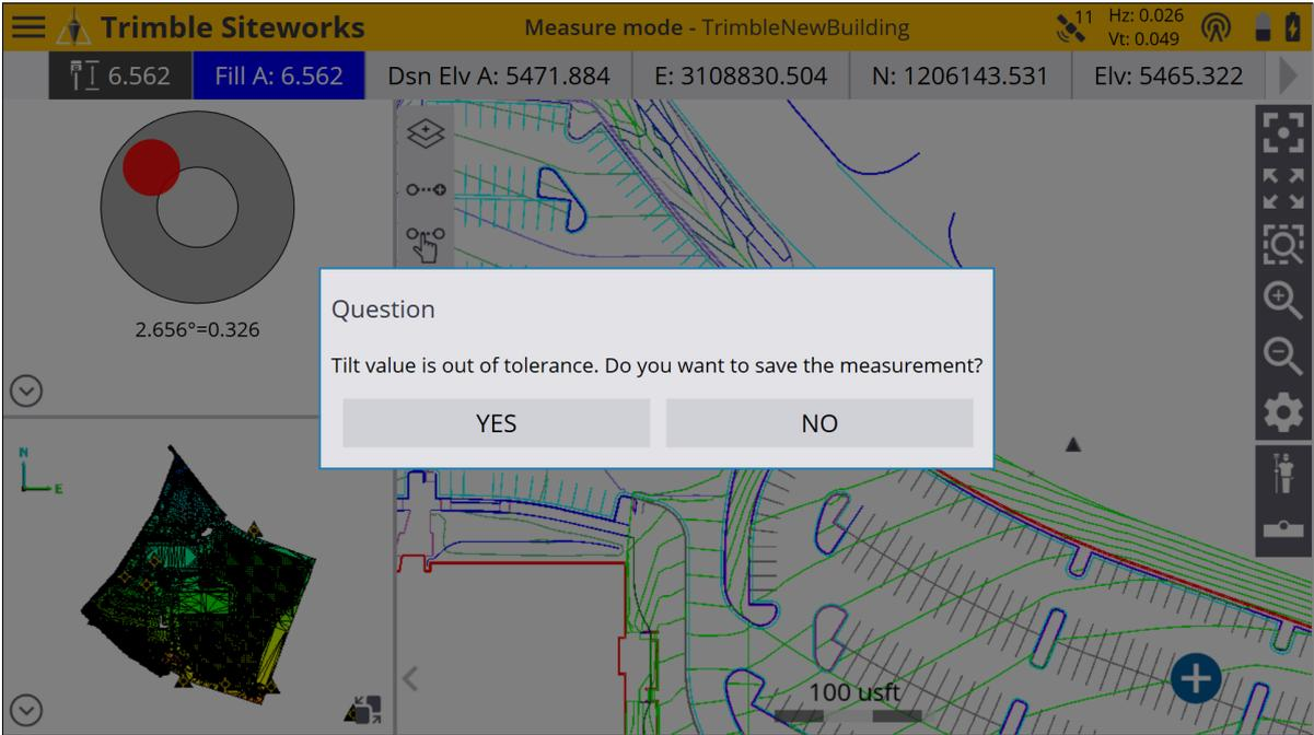
Tilt data are stored with each point measured with a compatible receiver and can be viewed by tapping-and-holding on a point and selecting **Point Information**, or by viewing point information via the Point Manager. The Tilt Angle, Tilt Error, and Tilt Tolerance values are stored. These tilt values are included in exported CSV data if the **Include QA data** option is selected.
