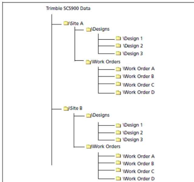
Work orders can be created directly in Siteworks or exported from the Business Center - HCE software. Creating a work order in Business Center - HCE allows for the assignment of the necessary design, surface offsets, measurement tolerances, instructions, coverage map grid size, and continuous measurement settings. Keeping data organized in work orders allows for easy import and data management within the Business Center - HCE software.
