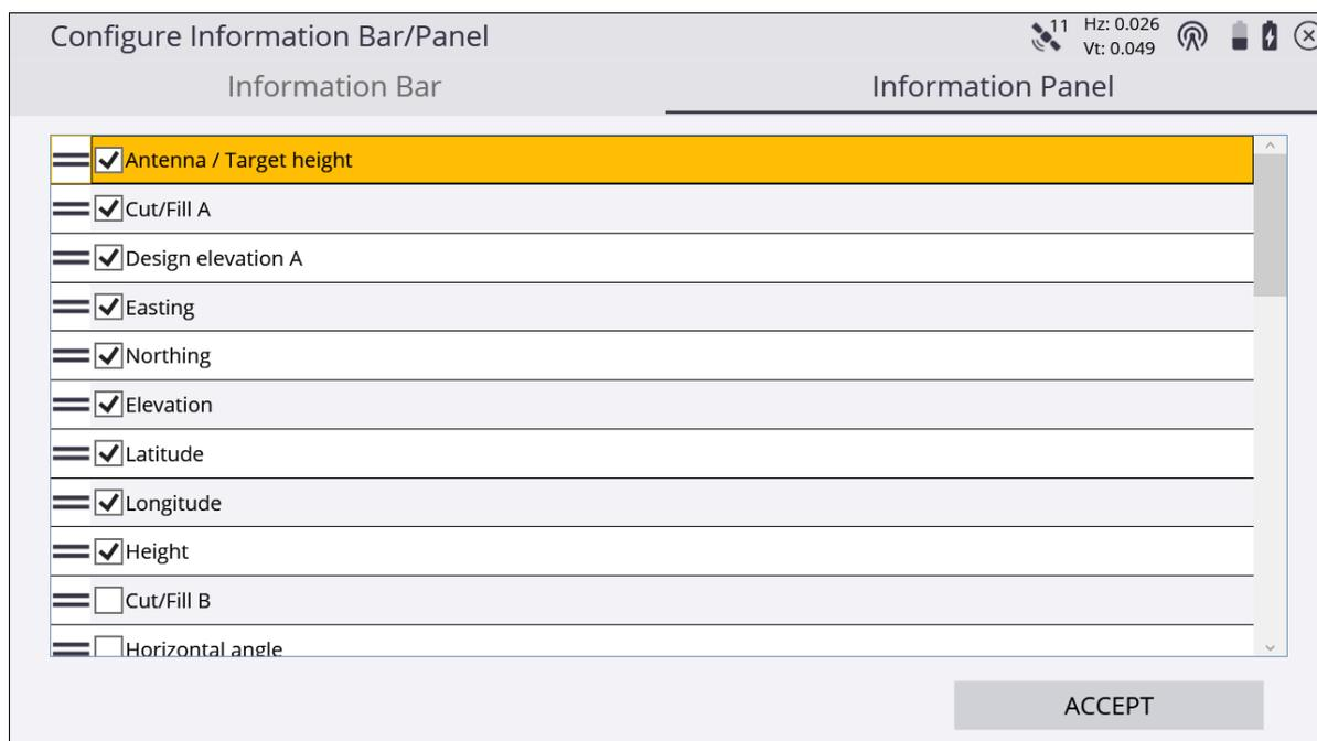
Some fields in the information bar (for example, Antenna & Target Height, Stakeout line offset, and Surface offset) are "active" fields. By tapping on it, you can change the settings and shortcut in the **Settings** dialog of this value. The active fields are indicated by white text on dark gray background.
