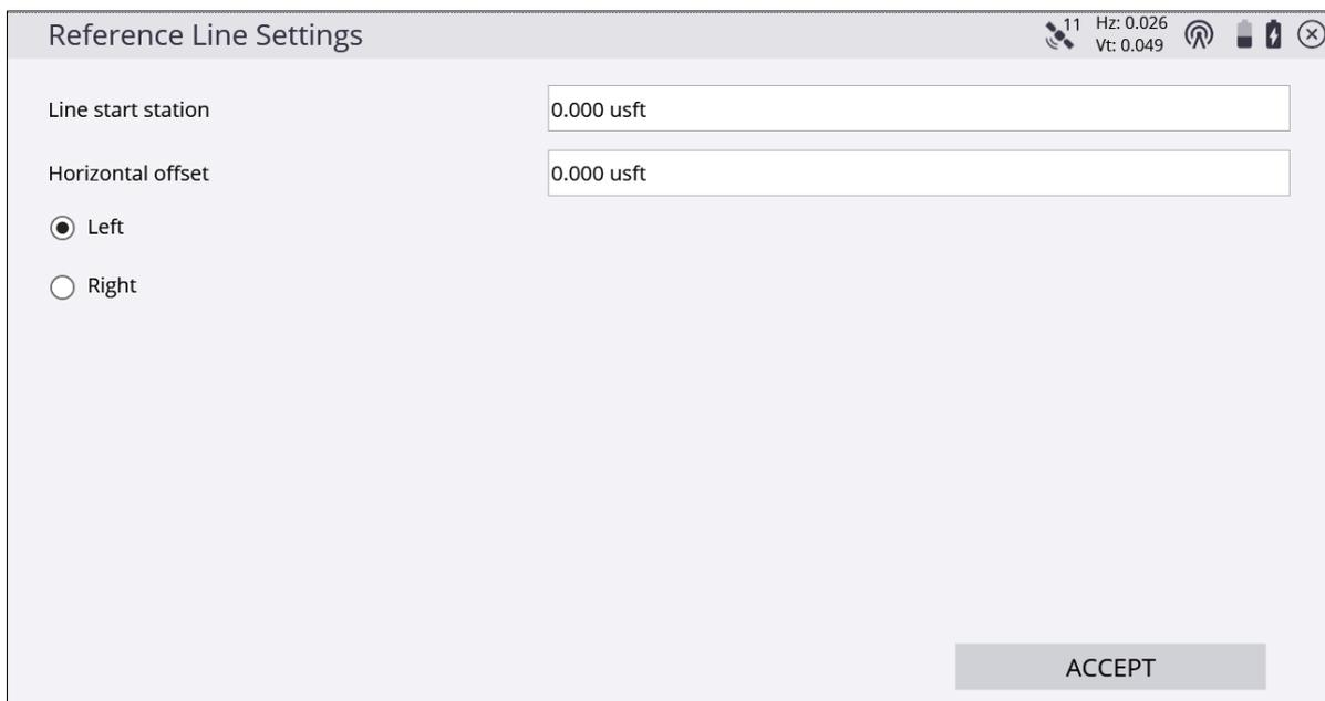
The image shows a screenshot of the 'Reference Line Settings' dialog box. The title bar at the top reads 'Reference Line Settings' and includes system icons for signal strength, battery, and a close button. The dialog contains two input fields: 'Line start station' and 'Horizontal offset', both with the value '0.000 usft'. Below these fields are two radio button options: 'Left' (which is selected) and 'Right'. At the bottom right of the dialog is a grey 'ACCEPT' button.
