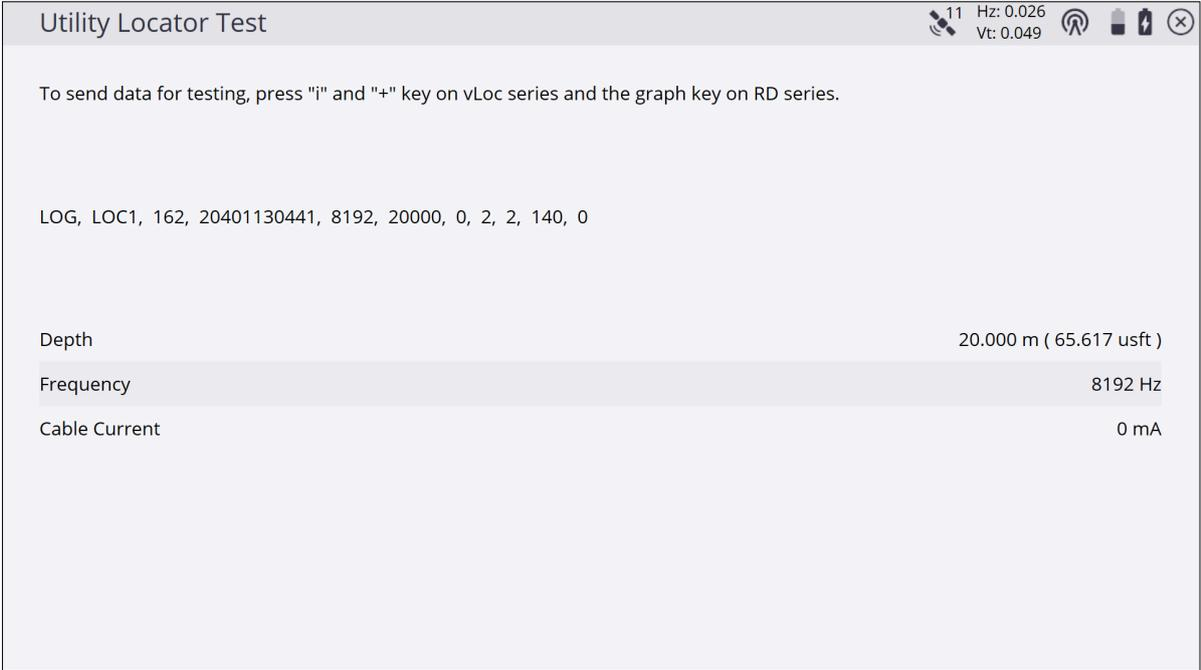
The screenshot shows the 'Utility Locator Test' screen. At the top right, there are status icons for signal strength (11), Hz (0.026), Vt (0.049), and battery level. The main text reads: 'To send data for testing, press "i" and "+" key on vLoc series and the graph key on RD series.' Below this is a data string: 'LOG, LOC1, 162, 20401130441, 8192, 20000, 0, 2, 2, 140, 0'. At the bottom, there is a table of test results:
