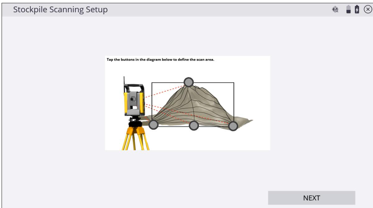
3. Define the shape of your stockpile. Start by tapping the gray dot at the highest point of the stockpile image on the screen.
