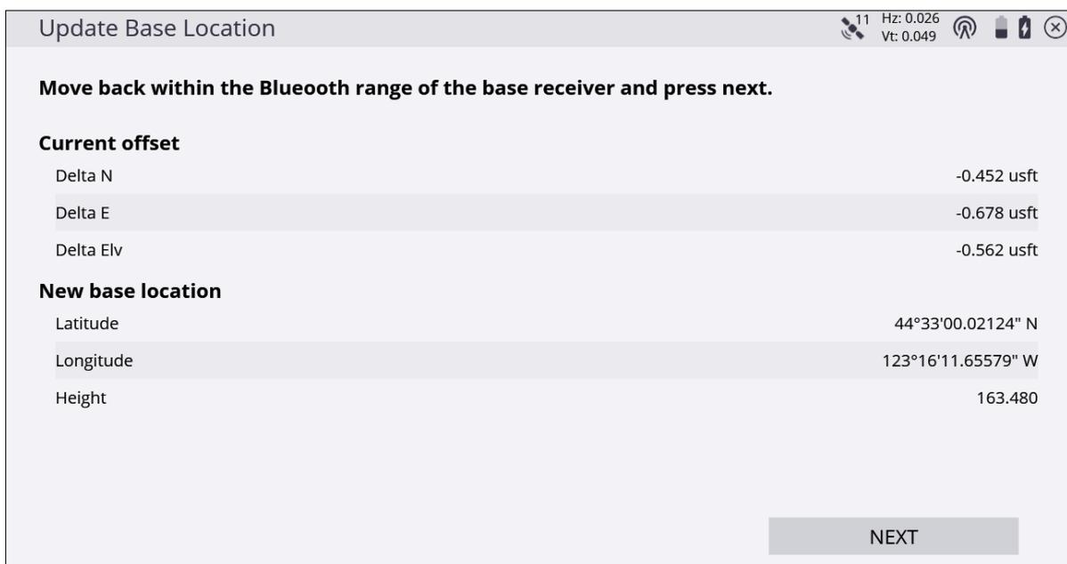
Updating the base receiver location this way enables the base, *while operating at its current location only*, to be used for machine control applications and by additional rover receivers on site, without having to perform Bench My Rover routines on each rover. If the
