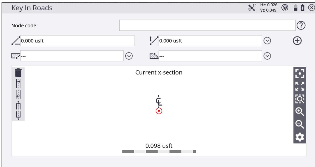
Pick the required station for the template. The following screen appears which allows entering the template.
