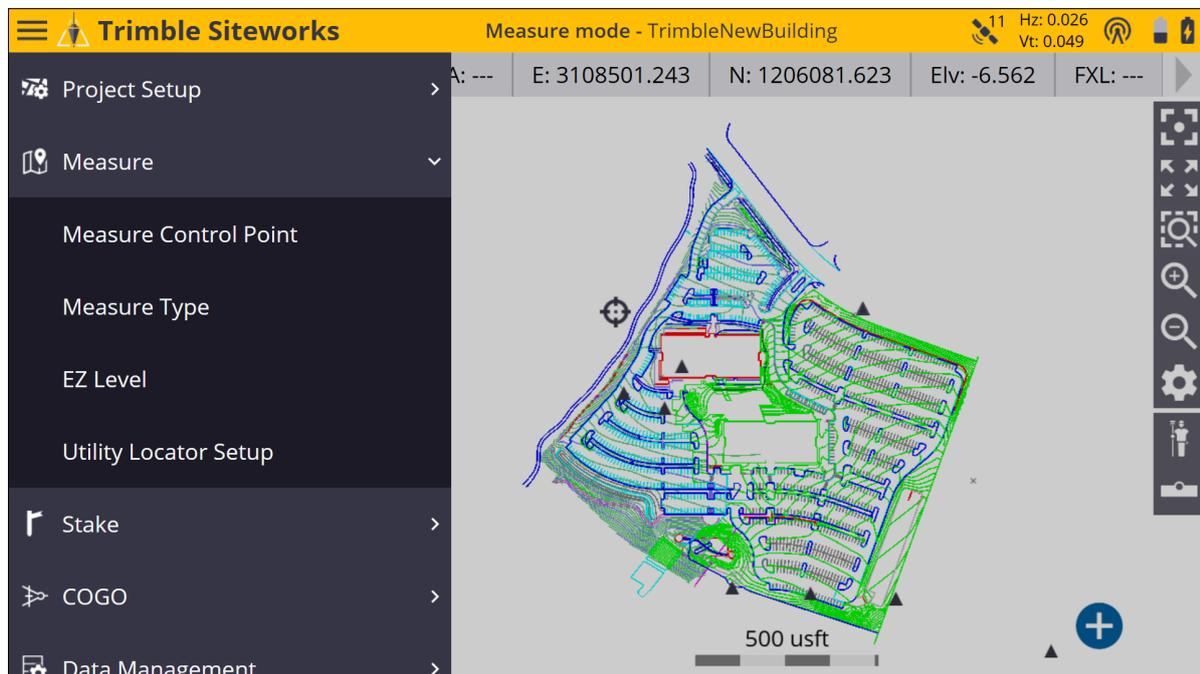
Tapping the **Utility Locator Setup** tab opens the **Utility Locator Setup** screen where the locator model, communication protocols, option for subtracting out the depth calculated by the locator are shown, in addition to enabling the connecting, disconnecting, and testing of the locator's output in Siteworks.
