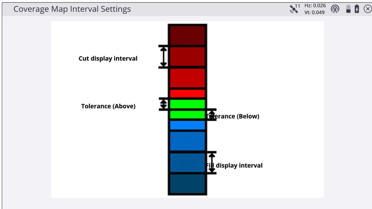
The Tolerance (Above/Below) value is how far above or below the design surface elevation the measured point can be to plot in a green, within tolerance color. The Cut/Fill display interval is the distance over which one color shade will be plotted. Different values can be set individually for the Cut and Fill display intervals, along with different individual Tolerance above and below values.
